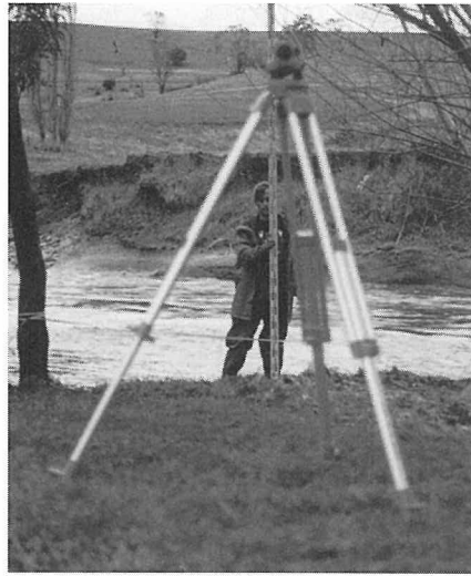
Setting levels for the hydrological survey.
